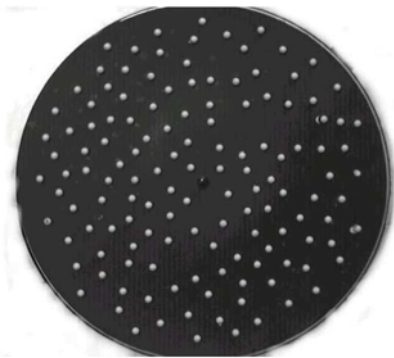
Fig. 2. Rotating disk for accuracy test of PIV S/W.
